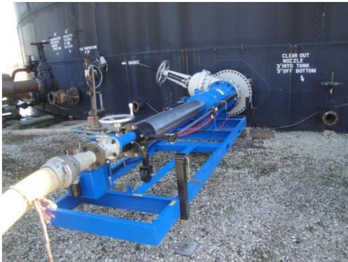
resuspension of the solids is finished and the recovered sludge is pumped off, the Hot Rod Twister is removed from the tank, and a regular Twister can be installed as a permanent fixture.
